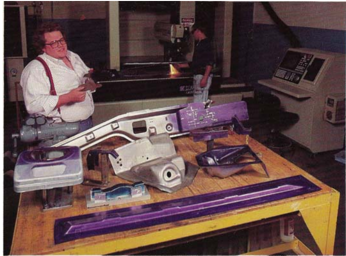
Auto Metal Craft's Kurt Woody (foreground) with an array of typical prototype parts. In the background is operator Joe Dewolf with the company's five-axis laser.
