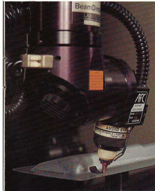
A five-axis laser can follow complex contours, remaining normal to the surface at all times. Automatic focus control brings accuracy and consistency to the cut, even with parts that exhibit high piece-to-piece irregularities such as stampings that spring back unpredictably.
