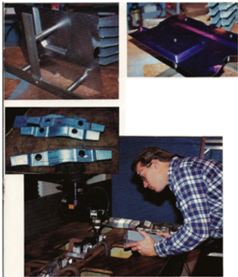
Laser operator Joe Dewolf uses the teach method to do basic programming on most parts, but often does subsequent editing to add detail. This part is typical.
